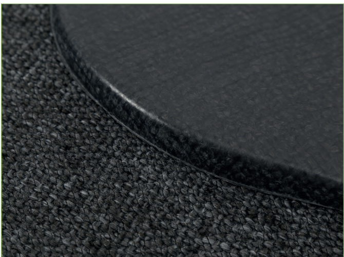
Fig. 4: Aesthetic part made of recycled carbon fibre
